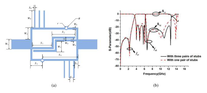
**Figure 5.** (a) The layout of proposed structure with additional stubs. (b) The compared results between the proposed structure with one pair of stubs and with three pairs of stubs.
