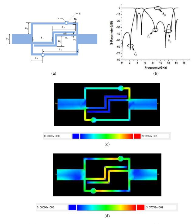
Figure 2. (a) The layout of first proposed loaded symmetric structure. (b) The simulated results of first proposed rotational symmetric loaded structure. (c) Current distribution at  $f_{z1}$  (2.32 GHz). (d) Current distribution at  $f_{z2}$  (8.56 GHz).
