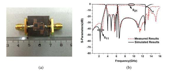
Figure 6. (a) Photograph of the fabricated circuit; (b) Comparison between the measured results and simulated results.
