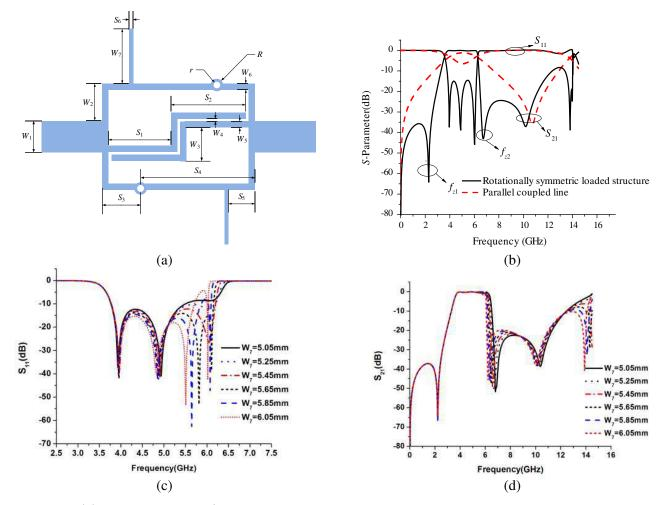
Figure 3. (a) The layout of  $\lambda/4$  parallel coupled line filter loaded rotational symmetric structure. (b) The simulated results of the  $\lambda/4$  parallel coupled line filter with/without loaded rotational symmetric structure. (c) The change pattern of inband modes when altering parameter  $W_7$ . (d) The change pattern of out-of-performance when altering parameter  $W_7$ .
